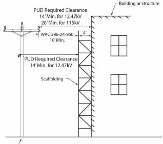
61. Please be advised that per WAC 296-24-960 the minimum worker safety clearance from any District distribution conductor is 10 feet. Therefore, the District requires a minimum 14-foot clearance from any structure to accommodate workers, scaffolding, and ladders.
