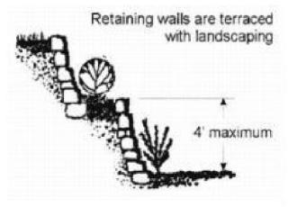
Response: All referenced retaining walls have been revised to 4' maximum. See sheet RD-02 for the updated wall and lot grading design. Specific retaining wall designs will be provided as part of the future grading permit submittal package.
