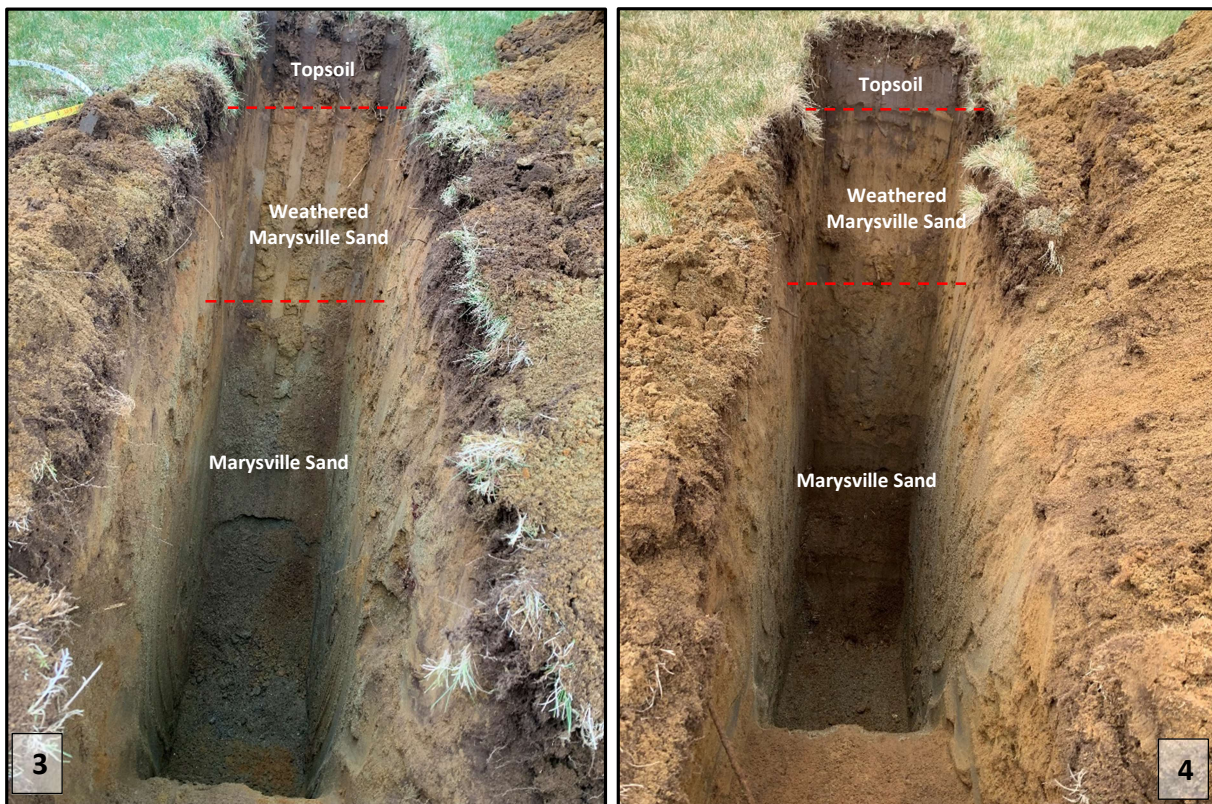
Images 3 and 4: General soil sequence observed in the test pits explorations where topsoil was overlying weathered Marysville Sand which was overlying non-weathered Marysville Sand (TP-1 – Image 3, TP-2 – Image 4).
