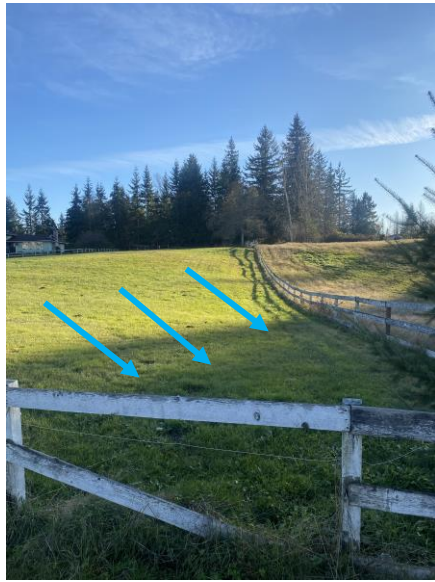
Image 3: Northwest property corner where runoff sheet flows west down existing slopes
