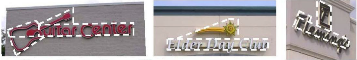
Figure 1: Wall Sign Area – Examples of Area Calculations
