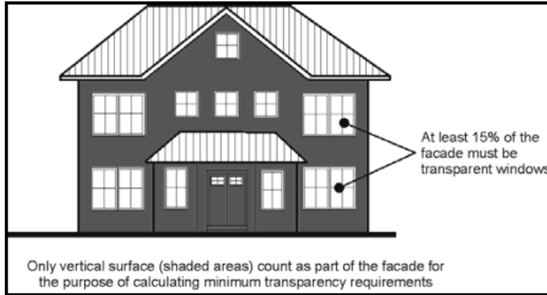
Figure 1 – Illustration of facade transparency requirements which enhance safety and the relationship to the street front.
