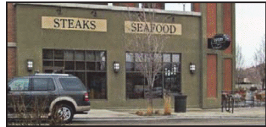
Figure 5 – For commercial buildings built up to the sidewalk, provide facade articulation features at no more than 30-foot intervals.
