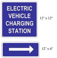
(2) Off-Street EV Parking – Parking Space with Charging Station Equipment. Combination signs identifying space as an electric vehicle charging station, prohibiting nonelectric vehicles, with charging time limits, should be provided, as depicted in Figure 7.
