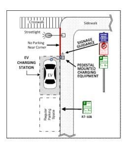
Figure 8: Electric Vehicle Charging Station – On Street
