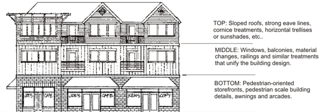
Figure 7-10. An example of clearly articulating a building's top, middle, and bottom by utilizing a combination of storefront elements on the ground floor, defined window patterns and articulation treatments on upper floors, and a distinctive roofline and/or top floor.
