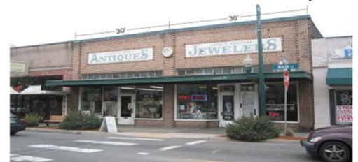
Figure 7-7. For commercial buildings built up to the sidewalk, provide facade articulation features at no more than 30-foot intervals
