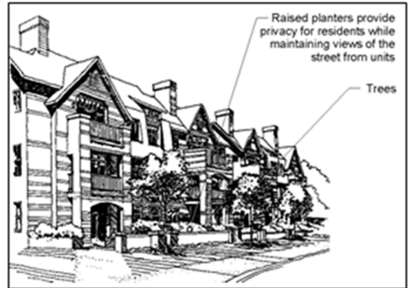
Figure 4-4. Multifamily building oriented towards the street.
