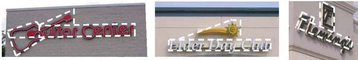
Figure 1: Wall Sign Area – Examples of Area Calculations
