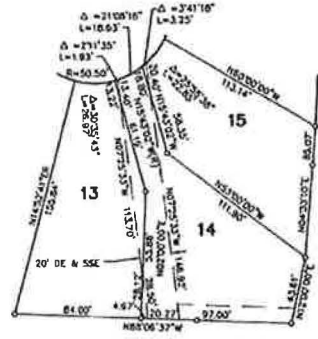
DETAIL OF 20' DRAINAGE & SEWER EASEMENT LOTS 13-15 SCALE 1" = 50'
