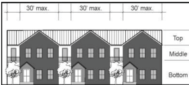
Figure B7 – Note the repeating distinct window patterns and the articulation of the building's top, middle and bottom.
