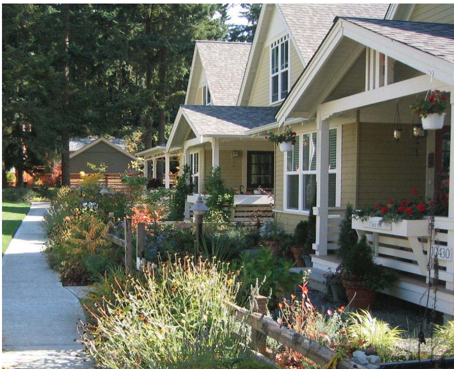
Figure B5. Note how the porches and the landscaping elements provide a graceful and inviting entrance transition from the public space to the private realm.
