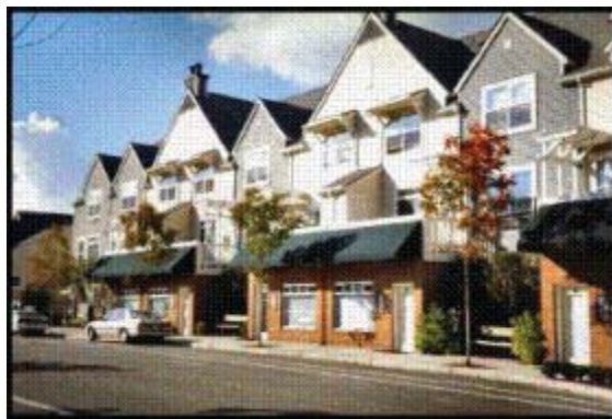
Figure C8 – This mixed use building incorporates decks, upper level setbacks, trellises, and landscaping to meet human-scale guidelines.
