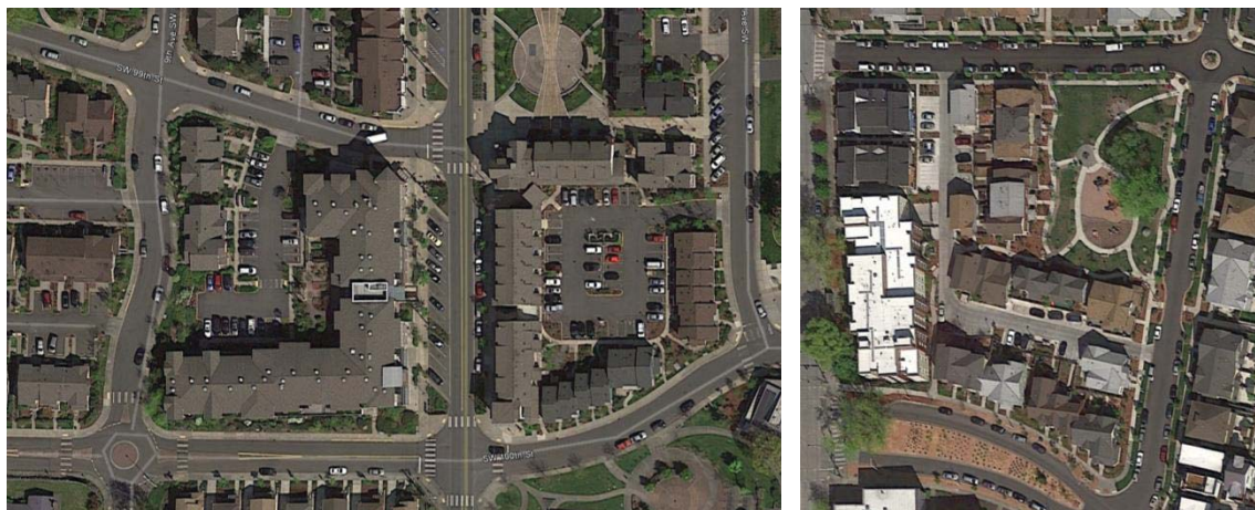
Figure C34. Examples of appropriately scaled mixed-use blocks that accommodate pedestrian connections no further apart than 300 feet.
