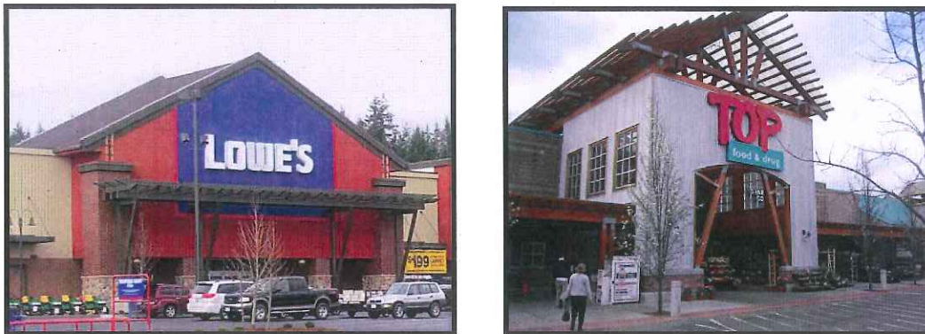
Figure 10 – Good examples of prominent pedestrian entries for large-scale retail uses. Note height change, vertical modulation, use of building materials, colors, and detailing to add interest and emphasis.
