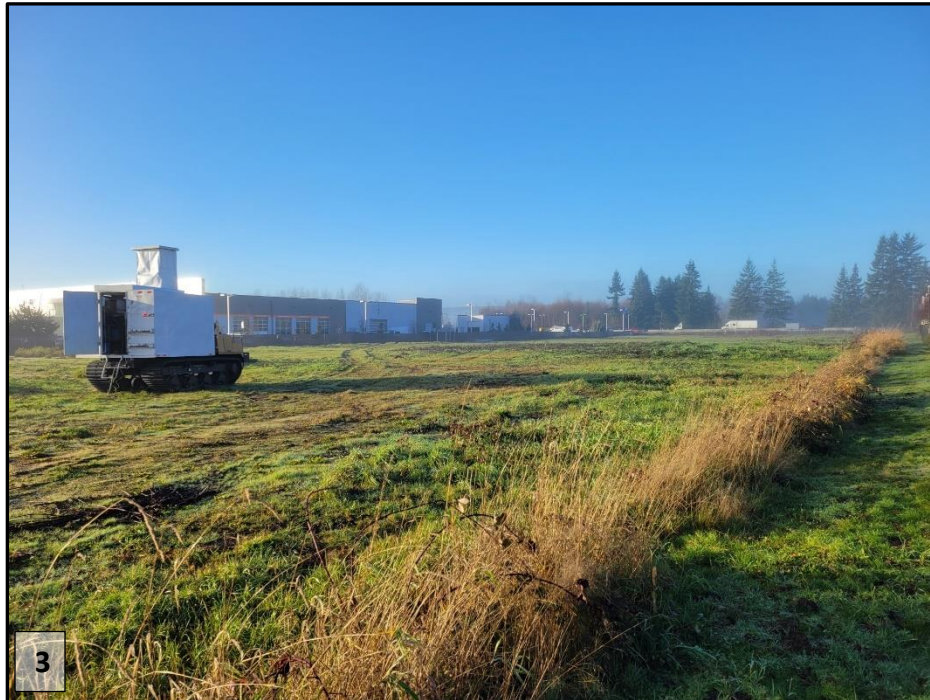
Image 3: A track mounted CPT machine, pushing exploration CPT-1, facing southwest.
