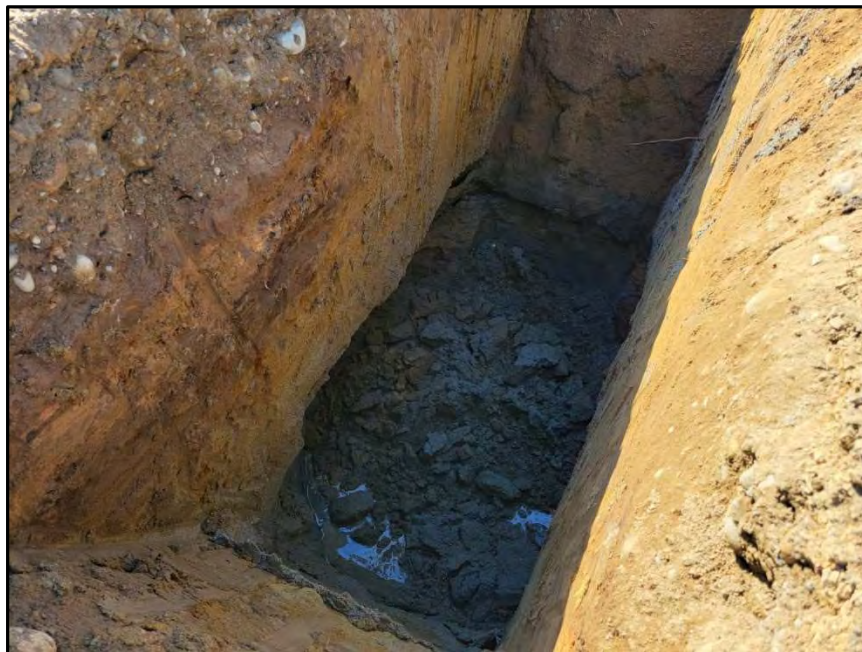
Image 2. Surface conditions within TP-1. Near-surface soils consist of gray gravel fill overlying sandy gravel fill, relict topsoil, and weathered Marysville Sand that transitions to unweathered, brown Marysville Sand.
