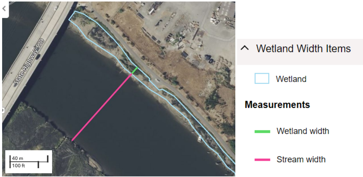
Figure 3-3. Width of Unit vs. Width of Stream
