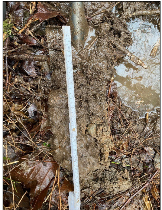
Photo 4: Soil Profile at DP-1W
