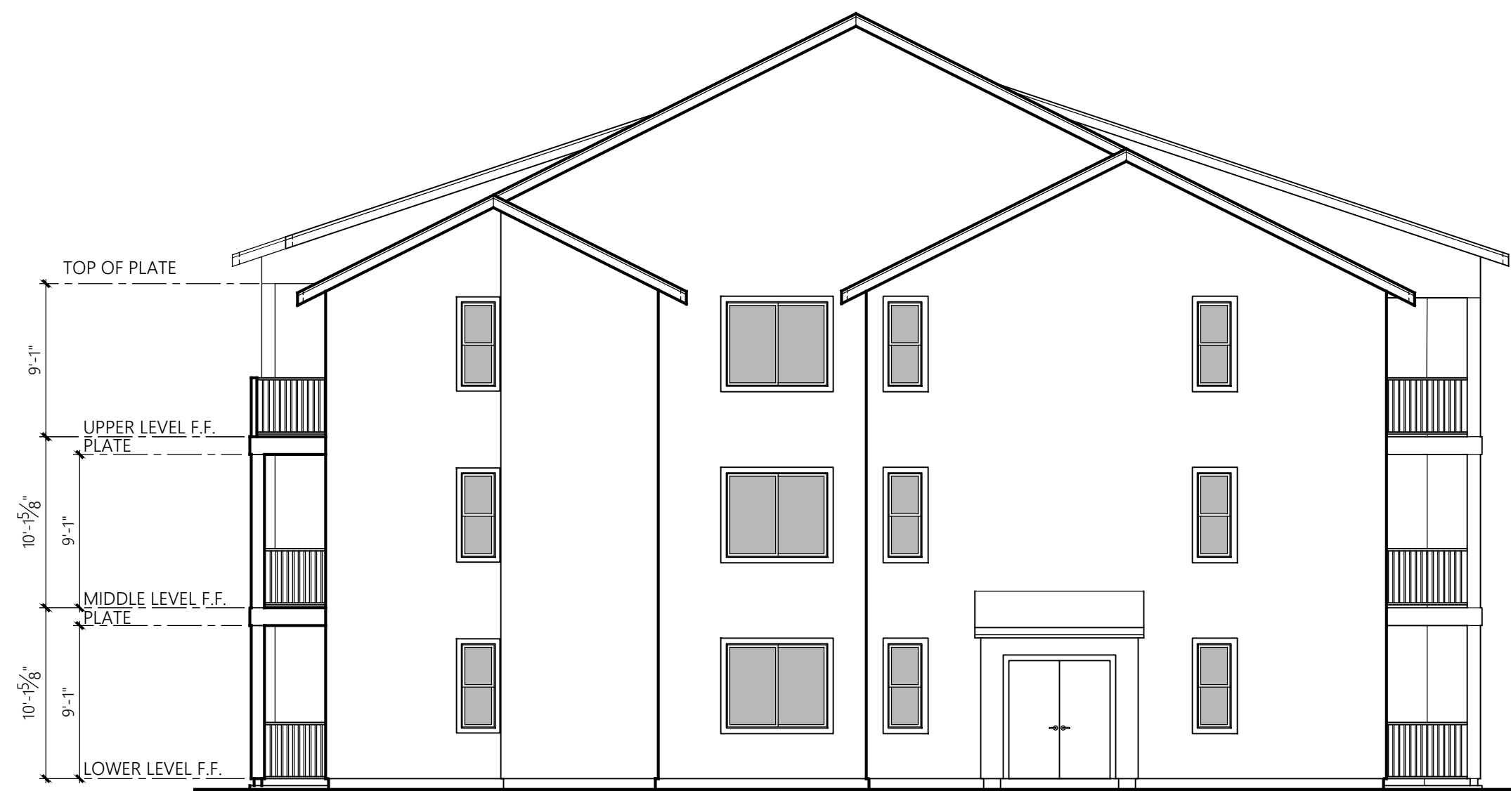
BUILDING TYPE 3 SIDE ELEVATION 1/8" = 1'-0"
