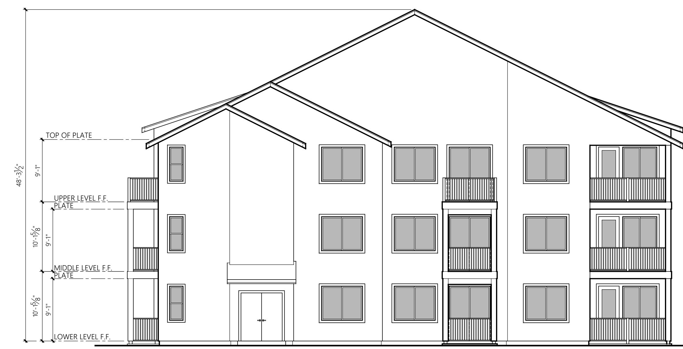
BUILDING TYPE 5 SIDE ELEVATION 1/8" = 1'-0"
