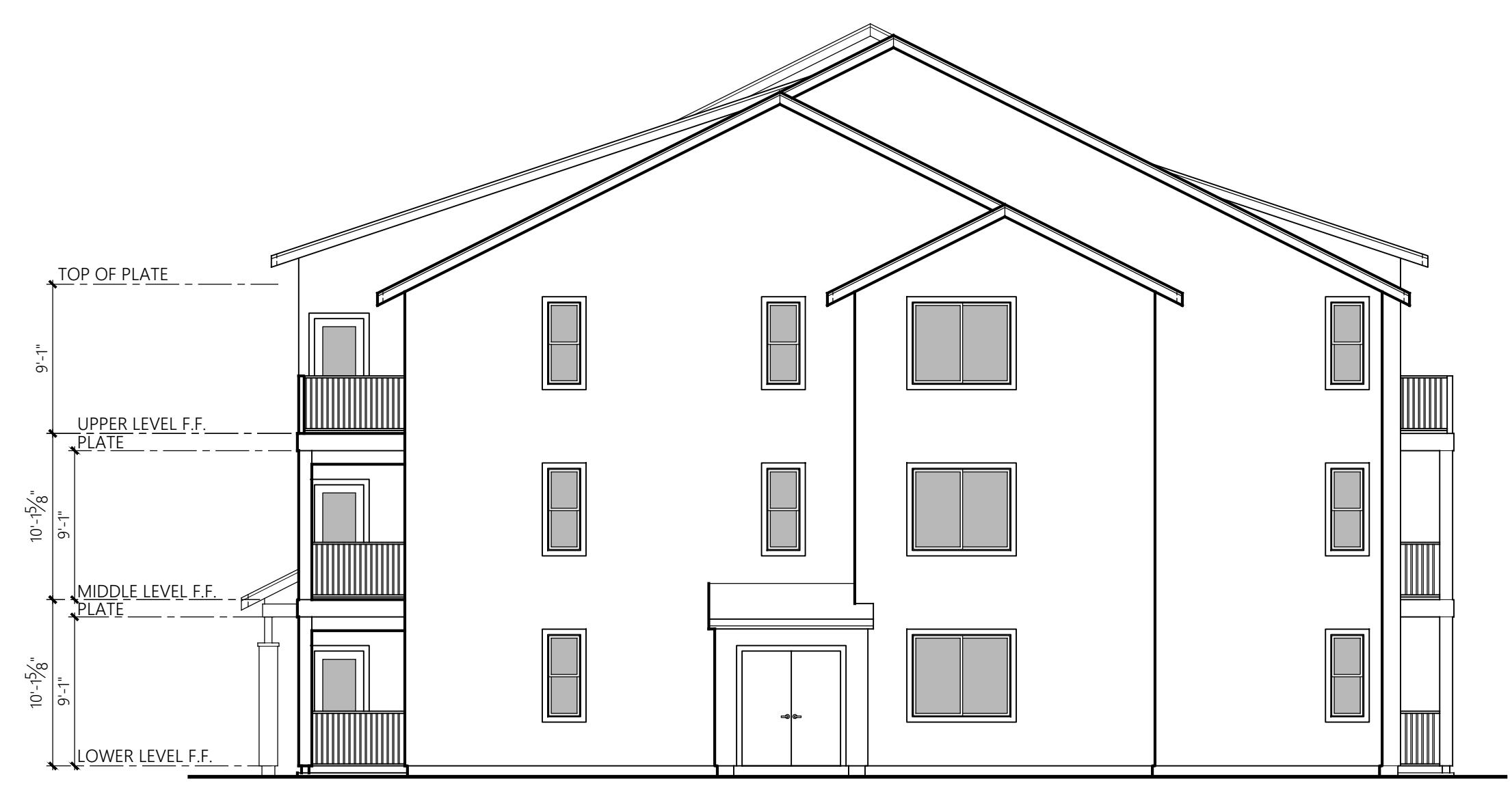
BUILDING TYPE 1 SIDE ELEVATION 1/8" = 1'-0"
