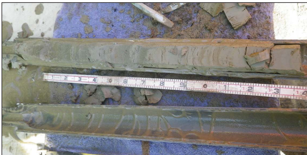
Figure 15. Surface of the glacial deposits from 55 to 56.5 fbs in B-9-17; top is left.
