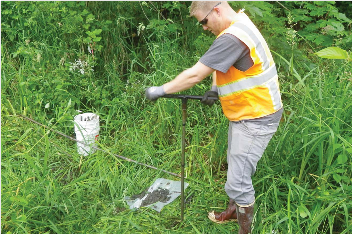
Figure 17. Hand augering at HA-1, view to the northwest.
