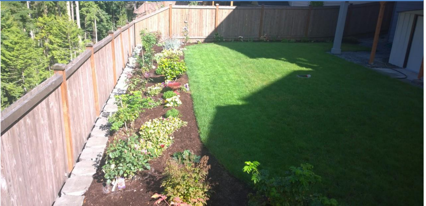
Figure 21-This is a backyard Recreation Storm Retention System as detailed in the schematic below it. This allows full typical use of the Backyard Private Space so important to these single-family homes. The backyard is fully functional while supporting a roof drain detention system that is twice filtered before being detained in the rock chamber below the turf grass.
