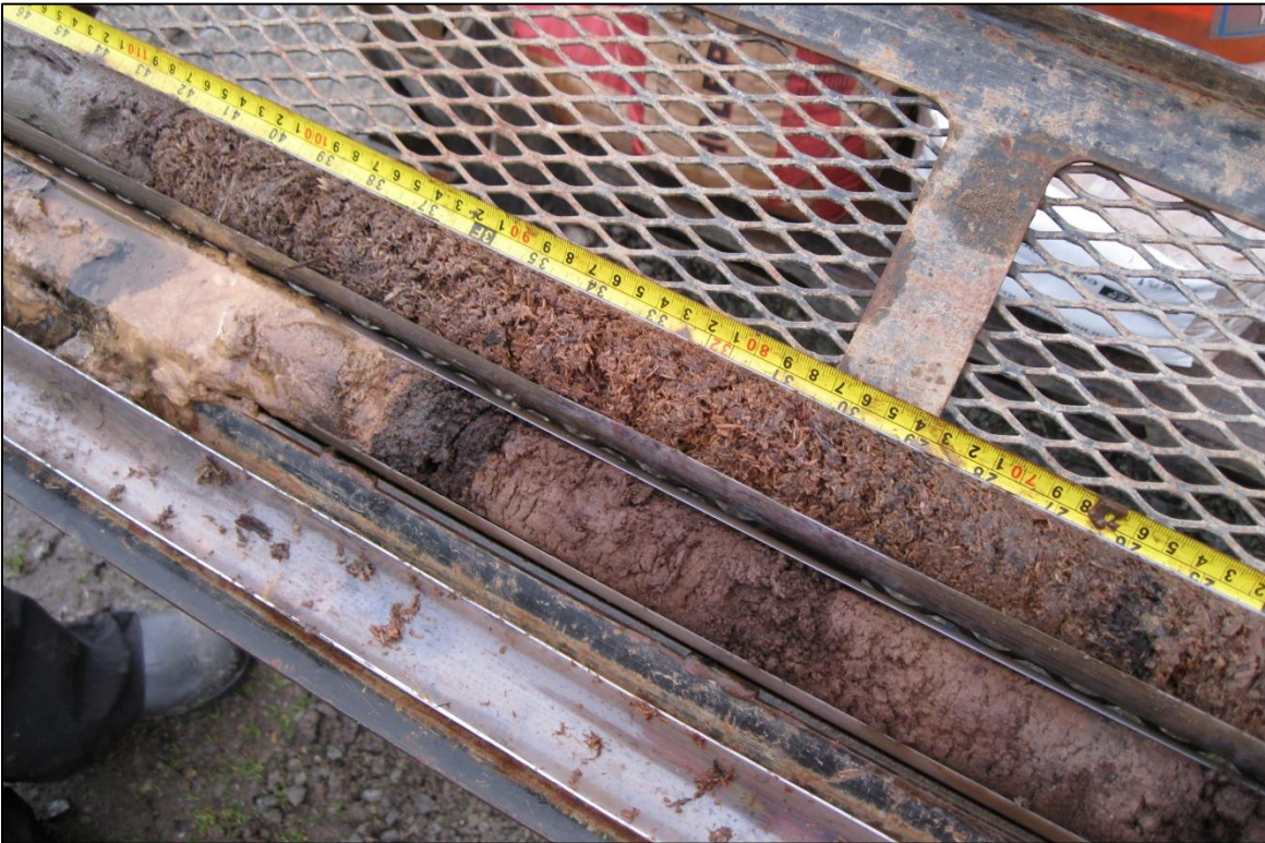
Figure 12. Photograph of sediments recovered within boring GM8 illustrating dominant woodchip/sawdust stratum encountered from 5-8 ft. (1.5-2.4 m) below surface.
