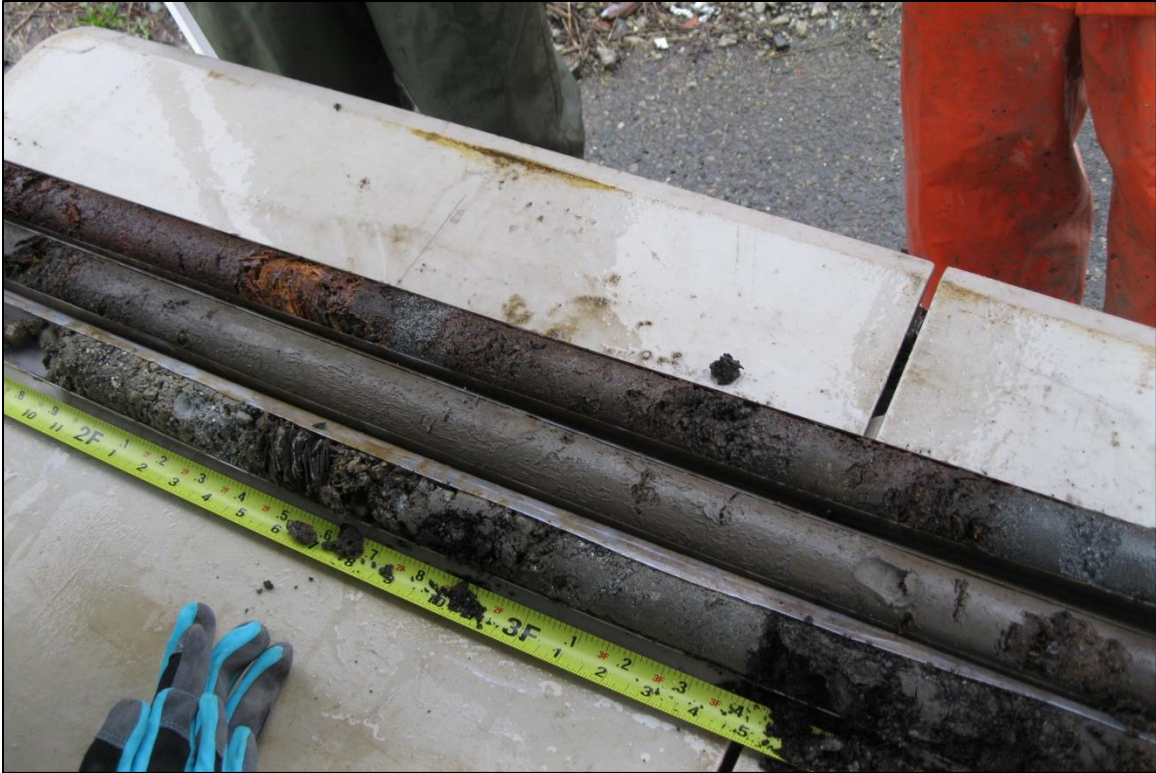
Figure 9. Photograph of sediments recovered within boring GM3; increasing depth left to right, bottom to top (each tube samples 5 ft.).
