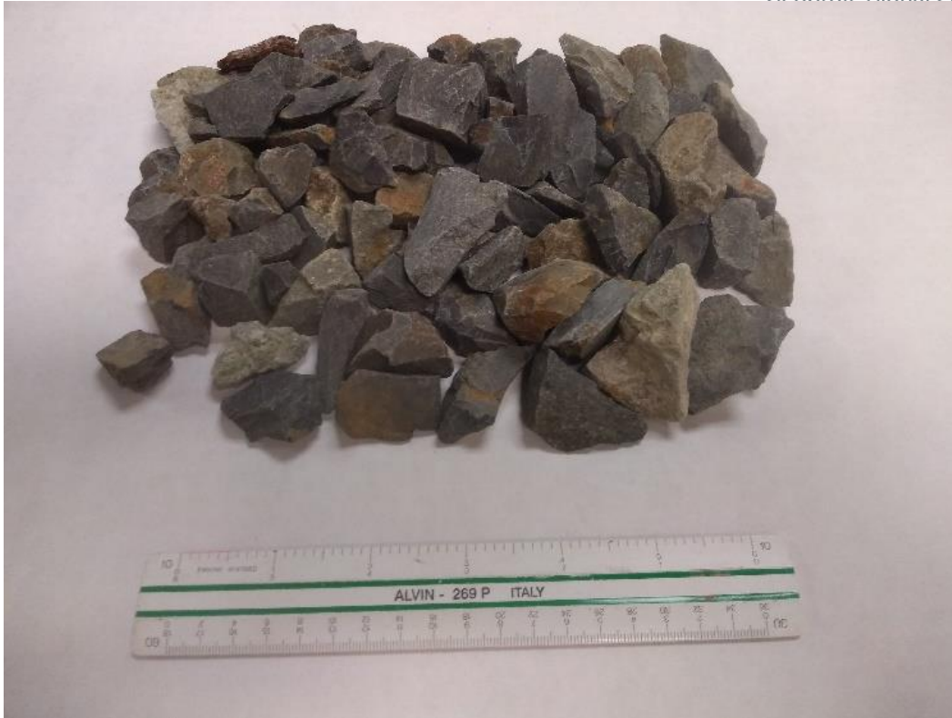
Iron Mountain Quarry “substation rock” used at the Fitzgerald Substation (Bothell, Washington)
