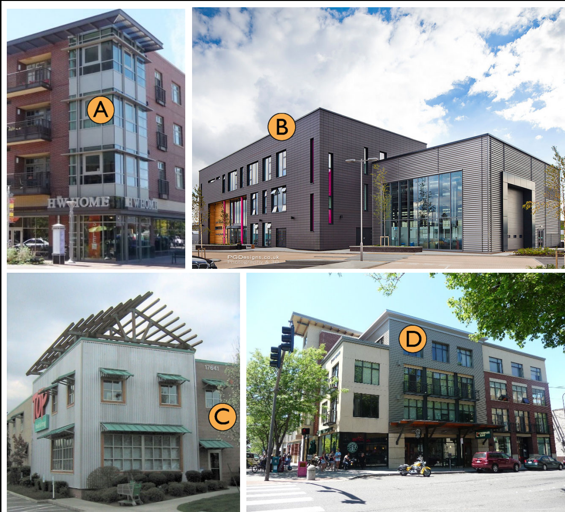
Figure 22C.080.530(2)(b) Acceptable metal siding examples
