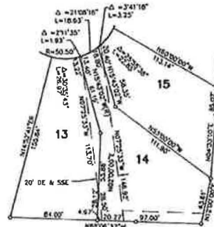
DETAIL OF 20' DRAINAGE & SEWER EASEMENT LOTS 13-15 SCALE 1" = 50'
