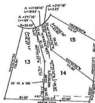
DETAIL OF 20' DRAINAGE & SEWER EASEMENT LOTS 13-15 SCALE 1" = 50'
