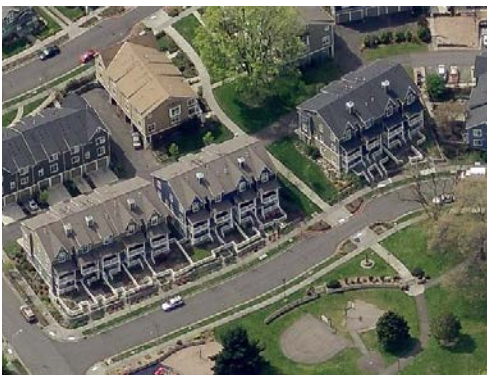
Figure 34. Well laid-out development with short intervals between pedestrian paths and a “green” path connecting to a park.
