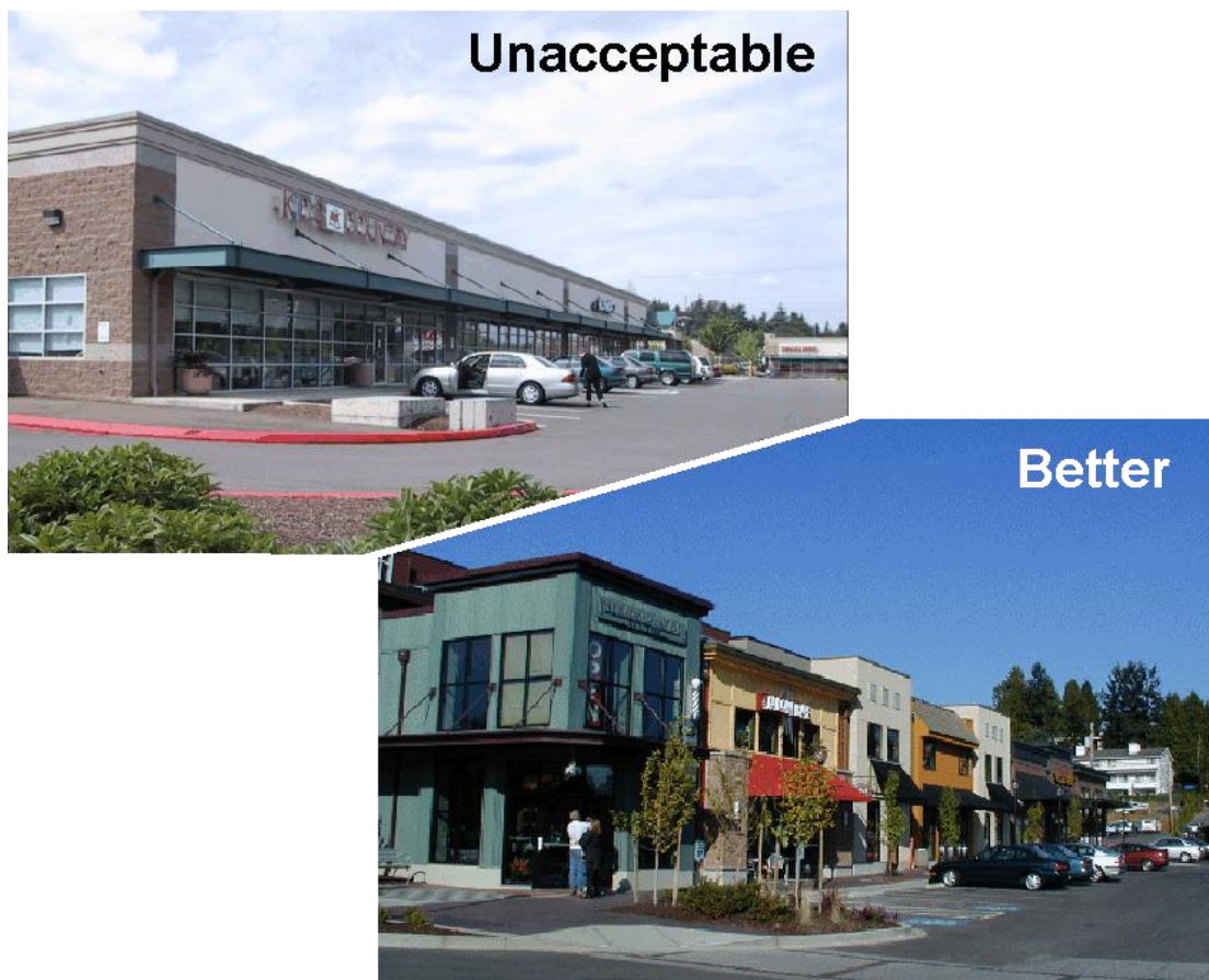
Figure C6. The continuous canopy on top is monotonous and deemphasizes individual storefronts. The bottom example provides a variety of weather protection features and represents a more desirable example.
