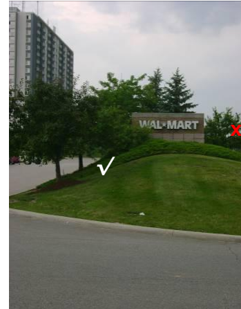
The height of a sign is measured from the grade of the street level where the sign is viewed; not from the top of the mound
