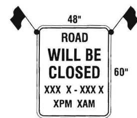
R11-1501 ADVANCED NOTIFICATION SIGN 1 (ANI) TO BE PLACED BY STATE 5 DAYS PRIOR TO CLOSURE
