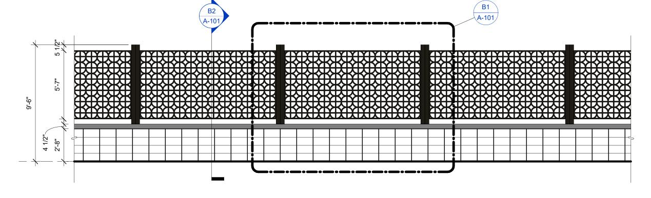
CAST CONCRETE COPING WITH DRIP EDGE (SLOPE 1/2" TOTAL), 48" LENGTHS, JOINTS TO BE SANDED SEALANT - 8" (NOMINAL) STACK BOND GROUND FACE CMU SOLID GROUTED - 1/2" EXPANSION JOINT MATERIAL, HOLD DOWN 1" AND FILL WITH SEALANT - FINISH SURFACE RE: CIVIL DRAWINGS COMPACTED SUBGRADE VERTICAL REINFORMENTRE: STRUCTURAL DRAWINGS HSS COLUMRE: STRUCTURAL DRAWINGS - CONCRETE FOOTING RE: STRUCTURAL DRAWINGS B2 LOW SCREEN WALL SECTION
