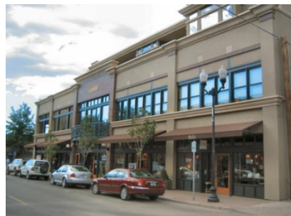
Figure 36 – Example of well-articulated building. Note how awnings, window divisions, pilaster columns, and cornice line all serve to divide up the façade into smaller segments without disrupting the unity of the overall design.
