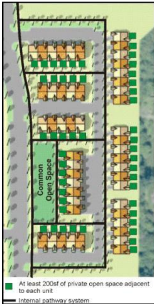
Figure 2019 - Example townhouse configuration with a combination of private open spaces adjacent to units and larger common open space accessible to all units.
